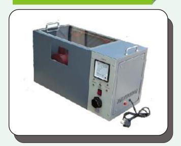
The oil cups are made of Acrylic & have removable electrodes for easy cleaning & polishing. The unique design of the lectrode holders eliminate oil leakages around shafts.
